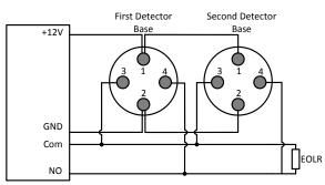
4-Wire Normally Open Wiring Diagram
