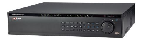
**DH-DVR3204LE-U:** 32 channel video inputs, 16 channel audio inputs, and 1 channel matrix output. The 1st, 9th, 17th and 25th video channels can support max D1(4CIF) realtime recording and other channels can support CIF realtime recording. It can support VGA, HDMI, eSATA, USB2.0 and 8 HDDs.
