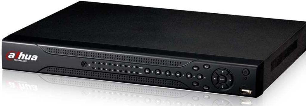
DH-DVR1604LE-A: 16 channel video inputs and 4 channel audio inputs. The 1st and 9th video channels can support max D1(4CIF) realtime recording and other channels can support CIF realtime recording. It can support VGA, HDMI and USB2.0.
