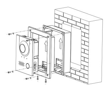
**Step1** Install the mounting box rear cover in the wall.
